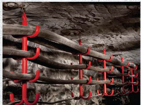
Strong, durable, extremely corrosion resistant for long life. Manufactured from high tensile spring steel, coated in thick, high dielectric grade, flame retardant PVC Plastisol.
