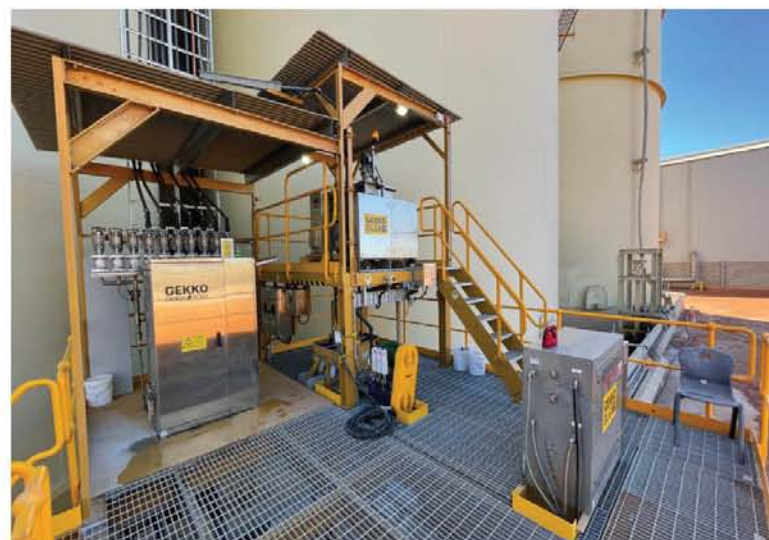
The Carbon Scout (left) and the Gekko OLGA (right) at Gruyere Mine in Western Australia.
